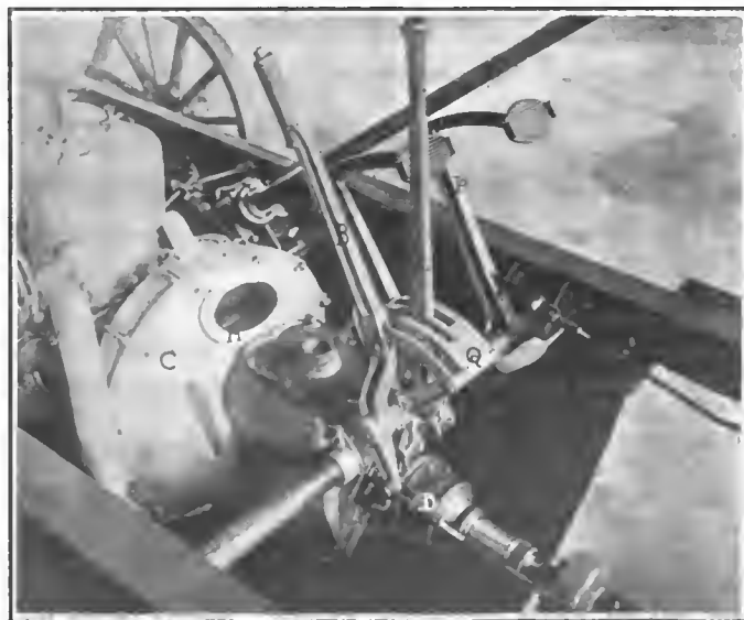
Fig. 7—View of flywheel and clutch housing. Note control levers in center
